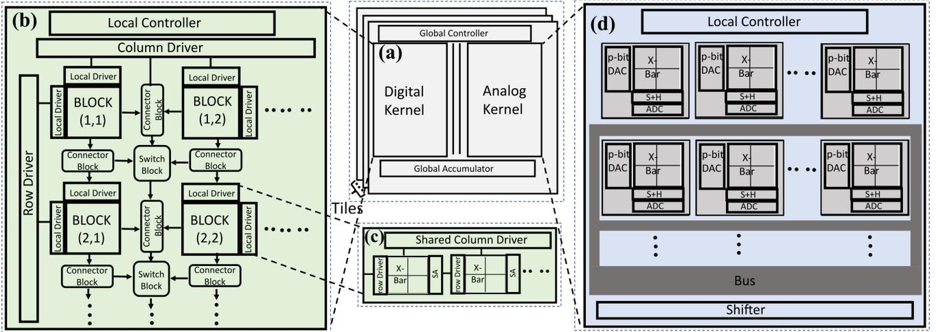
Fig. 9: Architecture overview of analog-digital hybrid accelerator.
