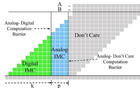
Fig. 5: Analog-digital barrier and analog-don't care barrier.
