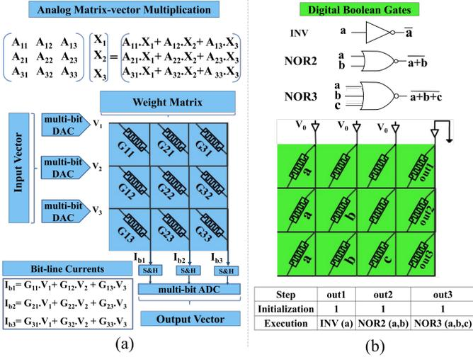
Fig. 1: (a) Analog in-memory computing using analog MVM and (b) digital in-memory computing using Boolean logic.
