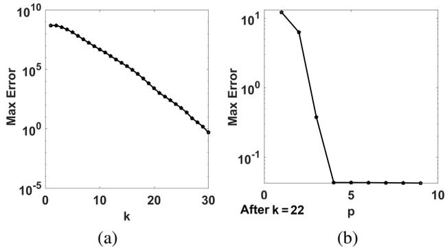
Fig. 6: The maximum error with respect to (a) the analog-digital barrier  $k$  and, (b) the analog-don't care barrier  $p$ . The experiment is performed using two 16 bit numbers.
