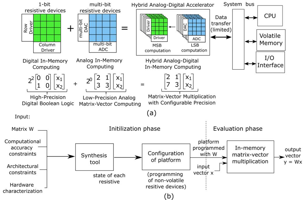
Fig. 2: Proposed hybrid in-memory computing platform .
