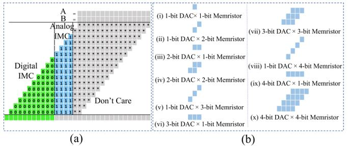
Fig. 7: (a) Analog-Digital-Don't Care covering problem and, (b) analog multi-bit multiplication cover library.
