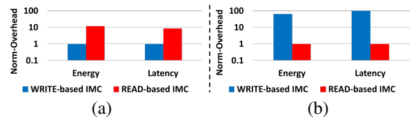
Fig. 3: Comparative energy and latency overhead for the systems in Fig. 2: (a) the Journals benchmark and (b) the GD99_c benchmark.
