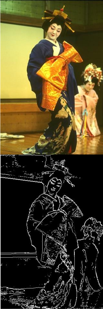
from edge detection using 8x8 ReRAM array.
